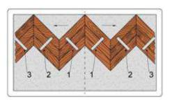
Start installing base elements from the center line along the wall farthest from the entrance. Do this by "dry" method - without fixing it with glue, to check the correctness and ensure accuracy before final fixing.
