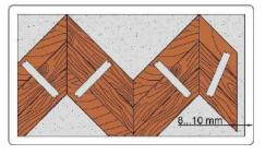
Use a protractor to determine the length and angle of the outer base element. Make sure that the length of the base element is sufficient to form an expansion gap after its installation.
