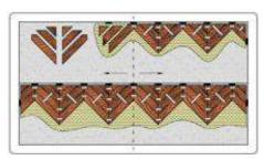
Install spacers along the wall to create a compensation gap. Apply glue to the base. Start laying the boards from the center line, alternating rows on both sides of it. Tap the boards with a mallet through the spacer so that the tongue of the board being installed fits tightly into the grooves of
