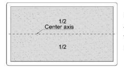
Divide the room in half lengthwise. Mark the center line using chalk line or a laser level to ensure accuracy. Check that the line is straight and aligned with the desired marks. If necessary, secure the line with a permanent marker.
