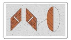
Assemble the basic elements from three planks (left+right). When assembling the basic elements, pay attention to the edges; the joints of the boards should be without protrusions.
