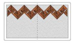
Make sure that base elements are laid out evenly and fit tightly together. Check the correctness of the installation and compensation gaps regularly. Make sure that everything is aligned and there are no distortions.
