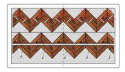
Using a straightedge set exactly at the tops of the inside corners of the first row of boards, draw a line with a marker. This will be the starting line after the boards are cut and laid into the overall covering. Number the boards to avoid mistakes when laying them out. Cut the boards along the markings. Use
